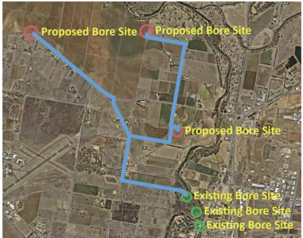
Figure 12 – Location of the Northern Bore Field Pipeline Project. The pipeline will be constructed within the road reserves of Bunglegumbie, Troy Bridge and Nulla roads as well as across Council owned land. From left to right, the names of the proposed production bores are Nevadon No. 2, Nevadon No. 1 and Sunnyside
