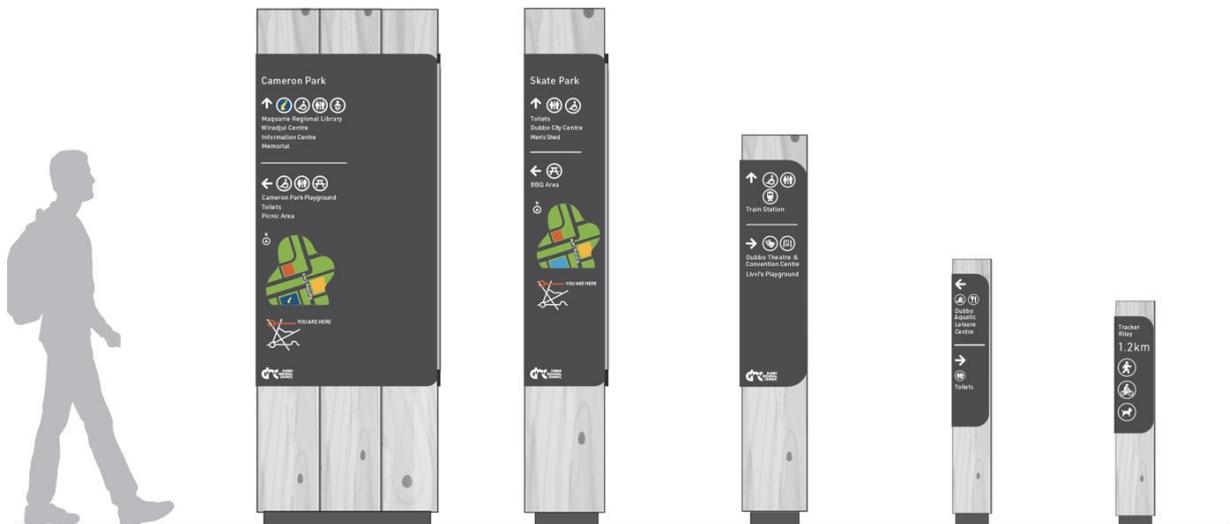
Figure 6. Architectural grade timber with Aluminium faceplate.
