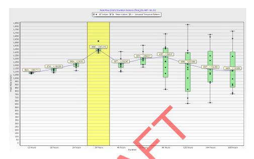
Figure C.7 Critical Temporal Pattern and Duration Assessment for 5% AEP Event (Critical Duration/Temporal Pattern Highlighted in Yellow)
