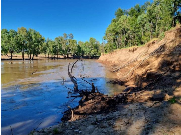
Photo 2: DMR\_R 28 – During site inspection in 2018 displaying gravel/cobble layers in bank toe.
