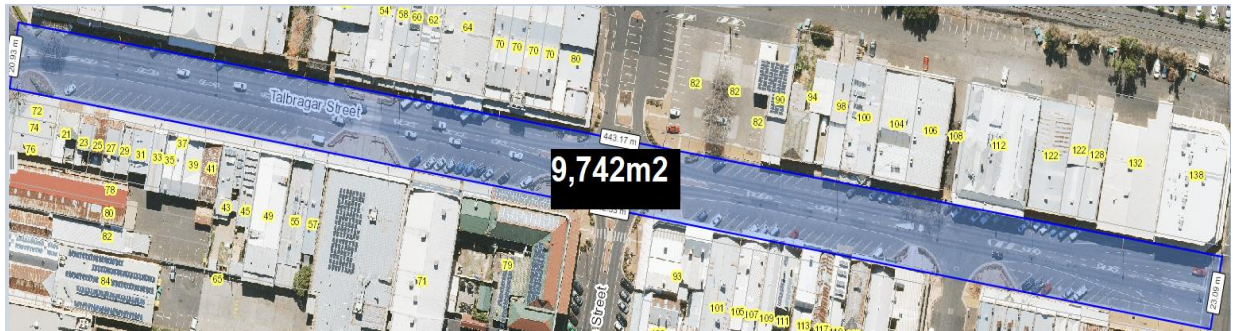
Figure 5. Hard surfaced area of Talbragar Street, totalling 9,740m 2 . Shaded area with tree planting, excluding existing trees, will be approximately 28% when trees reach full maturity.
