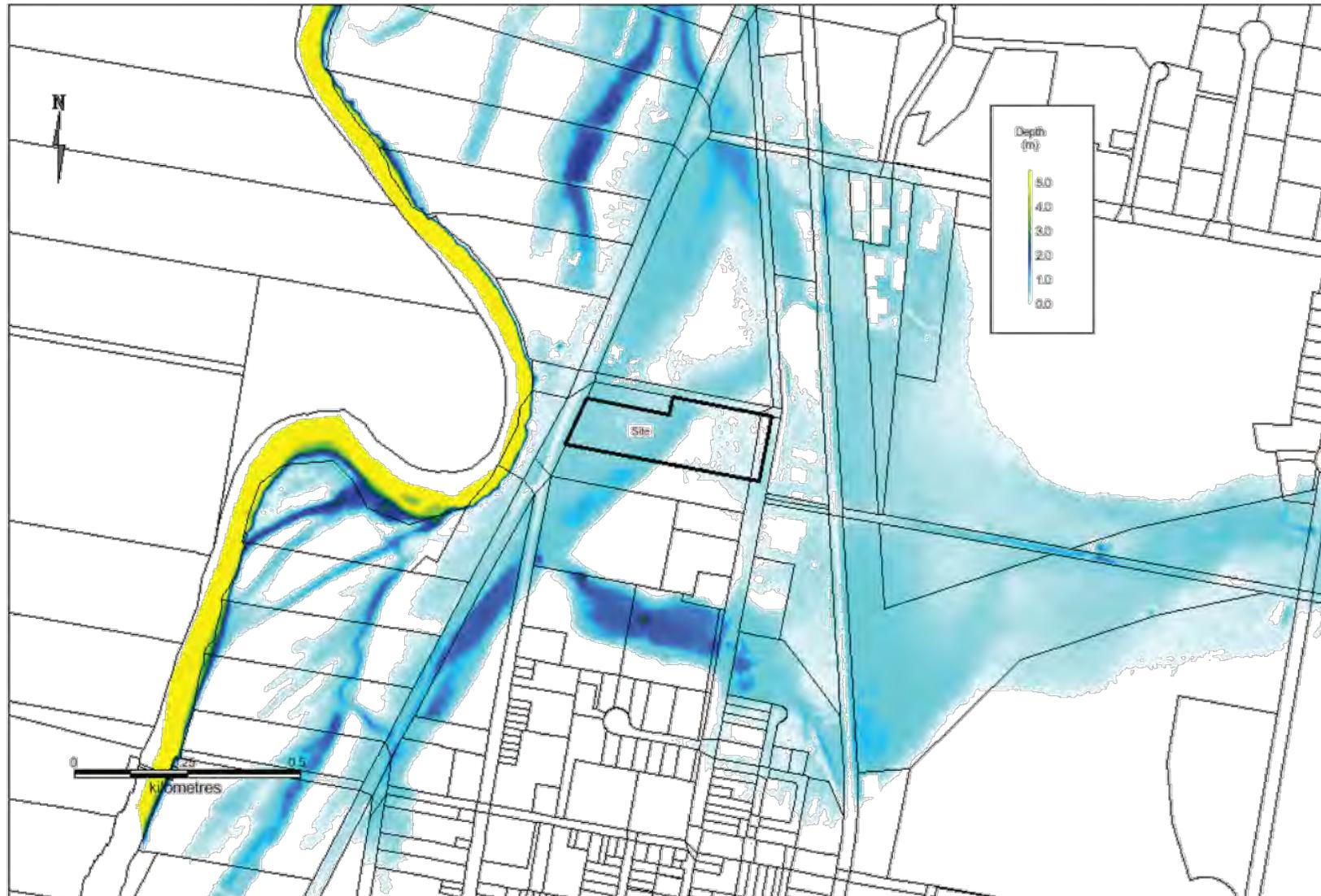
Figure 5 1% AEP Flood Depths – Troy Gully - Existing Conditions
