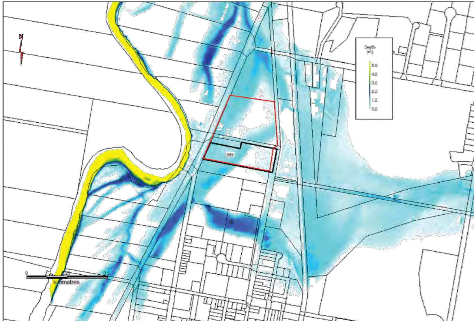
Figure 13 1% AEP Flood Depths – Troy Gully - Existing Conditions
