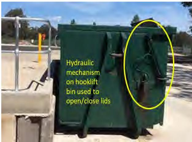
Hydraulic mechanism needs to be pumped up to open bins. A lever is used to release pressure and close bins. If residents are provided with keys to transfer stations they will need to be educated on how to use this equipment.
