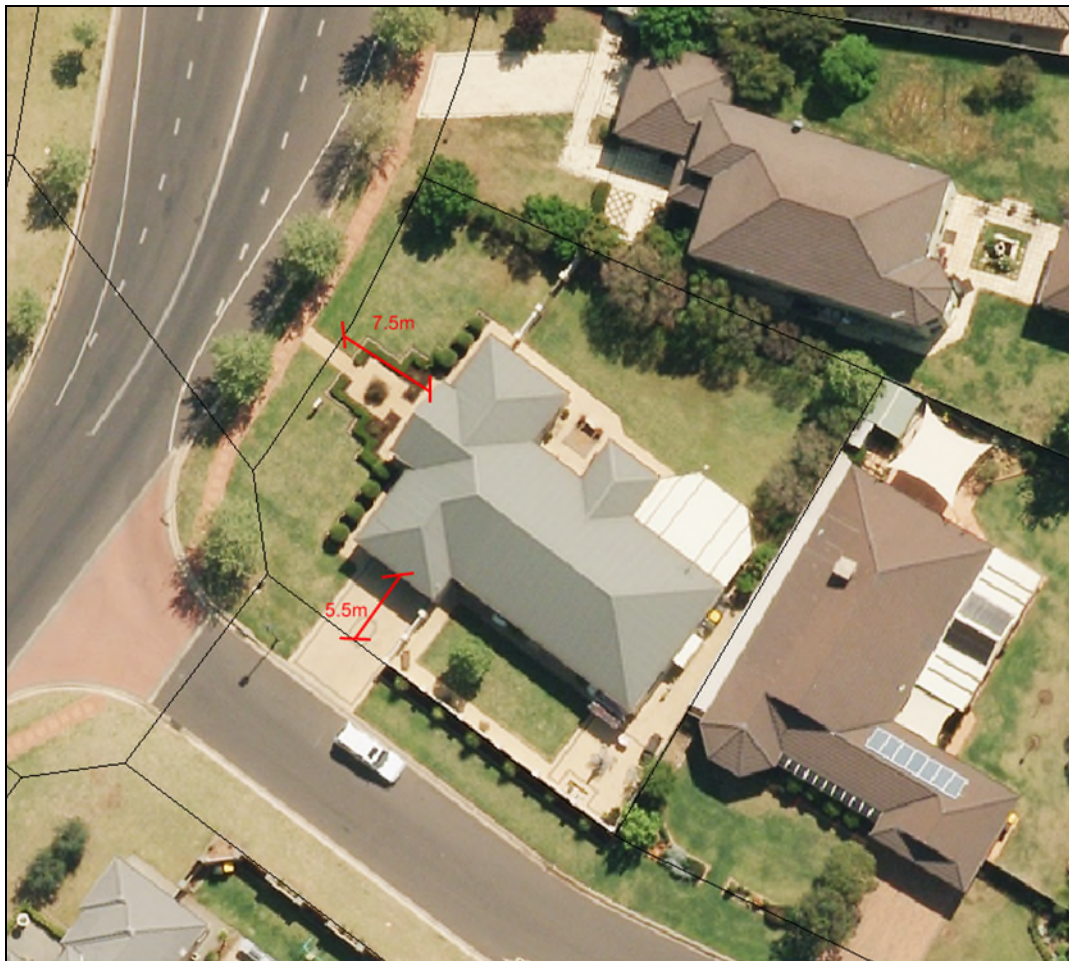
Figure 4: Corner allotment with the main entry to the primary road and the garage to the secondary road, with a set-back minimum of 5.5 metres
