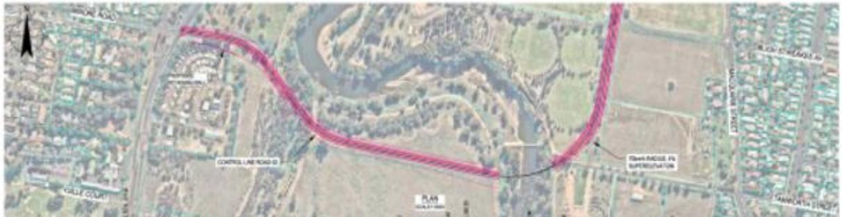
**Figure 4** – Option 4, identified as Option B in the GHD *Dubbo South New Bridge Strategic Concept Design Report*, attached as **Appendix 3**. Provides a connection from Whylandra Street at the Minore Road intersection on the west, to Bligh Street at the South Street and Sandy Beach Road intersection on the east. Estimated cost \$35,693,900.
