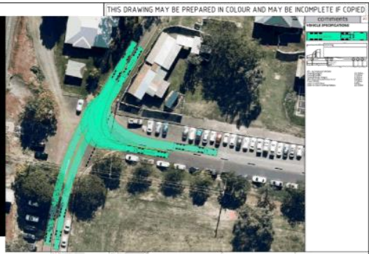
SEMI TRAILER SWEEP PATH FOR THROUGH MOVEMENT FROM MARY MACKILLOP TO MC GUNN DRIVE. ADVISED PATHWAY FOR MEDICAL GASSES ARTICULATED VEHICLES.
