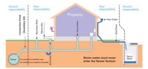
The yard gully is a fitting outside the home designed to release sewerage overflows safely. The shape and size of the yard gully can vary, but in general they are round grated drains between 100 mm and 150 mm in diameter.
