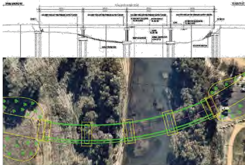
Figure 5-7 Superstructure Option 1 – Span arrangement on Road B
