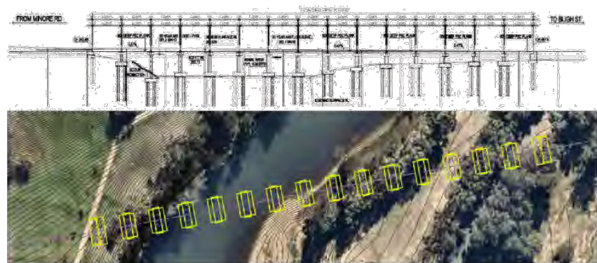
Figure 5-11 Superstructure option 2 – Span arrangement on road A
