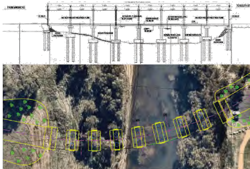
Figure 5-14 Superstructure option 2 – Span arrangement on road B
