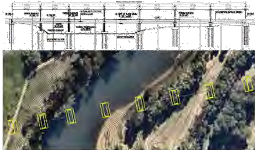
Figure 5-4 Superstructure Option 1 – Span arrangement on Road A
