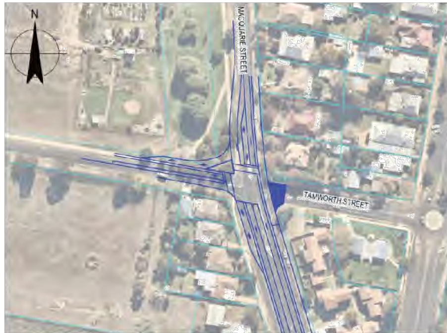
Figure 2-8 Proposed intersection details at Macquarie Street / Tamworth Street intersection detailing no entry / exit via Tamworth Street east of Macquarie Street
