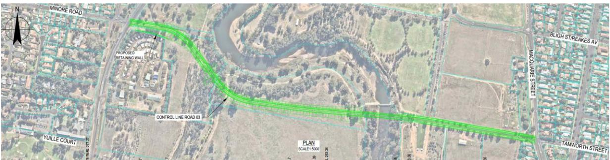
**Figure 2** – Option 2, identified as Option C in the GHD *Dubbo South New Bridge Strategic Concept Design Report*, attached as **Appendix 3**. Provides a connection from Whylandra Street at the Minore Road intersection on the west, to Macquarie Street at the Tamworth Street intersection on the east. Estimated cost \$39,049,900.
