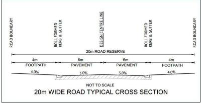
Figure 3: Cross-section of the 20 metre road reserve
