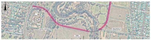
**Figure 4** – Option 4, identified as Option B in the GHD *Dubbo South New Bridge Strategic Concept Design Report*, attached as **Appendix 3**. Provides a connection from Whylandra Street at the Minore Road intersection on the west, to Bligh Street at the South Street and Sandy Beach Road intersection on the east. Estimated cost \$35,693,900.
