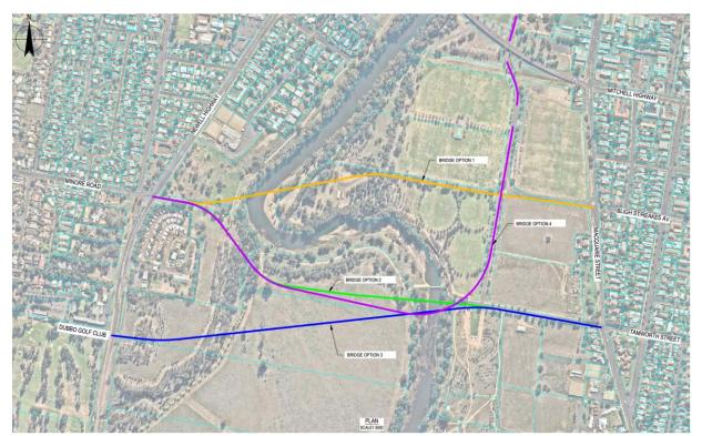
**Figure 5** – Options 1, 2, 3 & 4 and their comparative alignments. See the GHD *Dubbo South New Bridge Strategic Concept Design Report*, attached as **Appendix 3** for further details.
