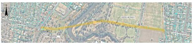
**Figure 1** – Option 1, identified as Option A in the GHD *Dubbo South New Bridge Strategic Concept Design Report*, attached as **Appendix 3**. Provides a connection from Whylandra Street at the Minore Road intersection on the west, to Macquarie Street at the Bligh Street and Reakes Avenue intersection on the east. Estimated cost \$41,402,300.
