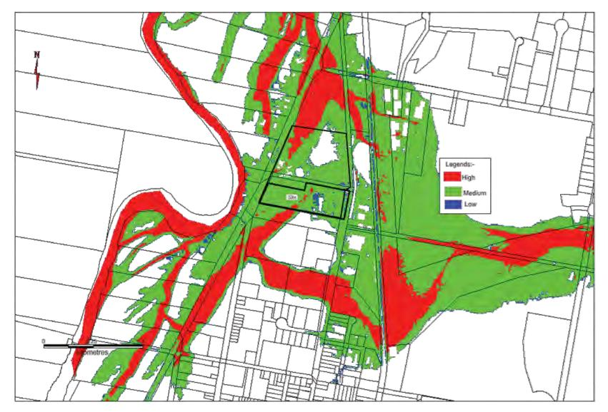
Figure 16 1% AEP Flood Hazards - Troy Gully - Existing Conditions
