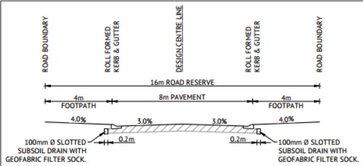
Figure 3: Cross-section of the 16 metre road reserve
