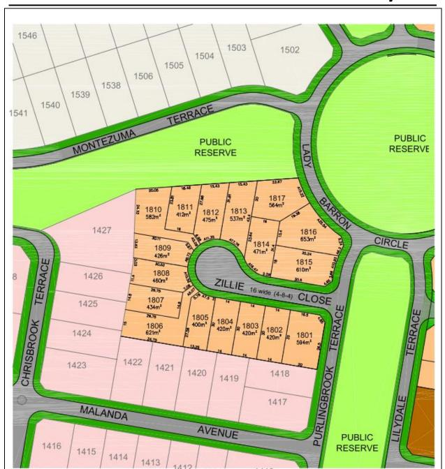
Figure 2: Road layout to be constructed as part of Development Consent D2021-372 – Stage 18 - Zillie Close. Please note the other road names shown on this map have been approved and gazetted and not part of this report.
