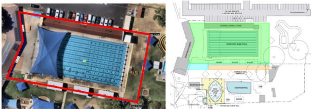
Figure 2. Existing DALC and a schematic showing extent of works involved in enclosing the 50-metre pool (green).
