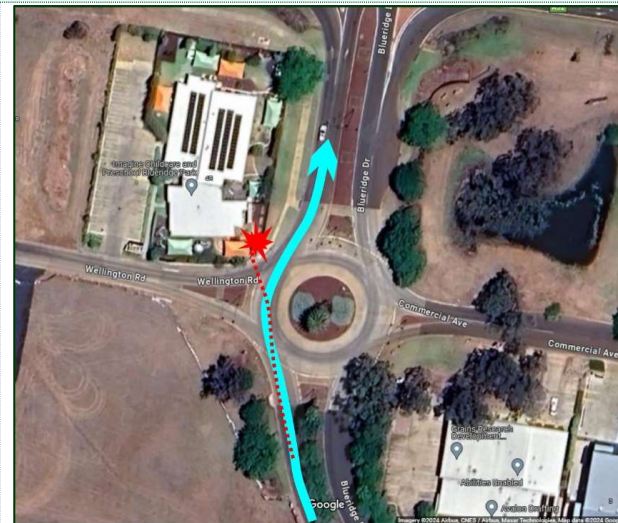
F1.2: Aerial photograph of the roundabout and southern approach. Blue arrow, straight through on Blueridge Dr, Red dotted line potential path of an off-road crash. (Aerial photograph: Google Maps)
