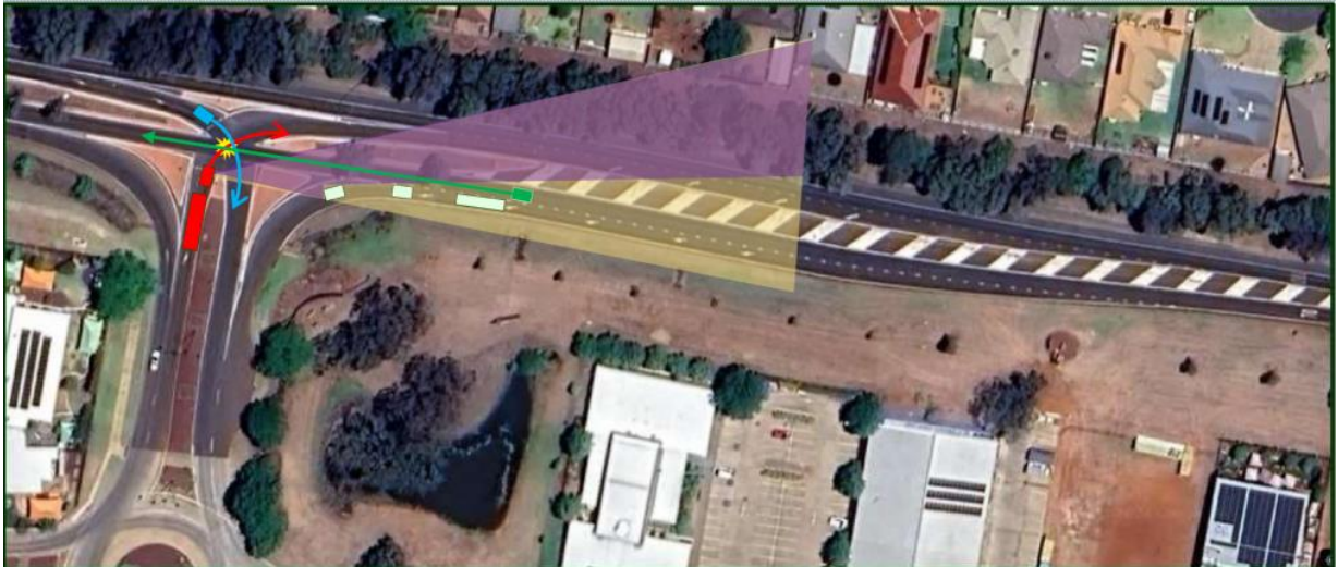
Figure 9: Visual representation of sight line limitations and potential crash types at the Mitchell Highway seagull intersection
