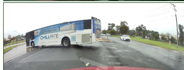
F4.2: Bus driver selecting a small gap, requiring through vehicles to slow to avoid a collision, with potential for queueing of through vehicles across the Children's Crossing.
