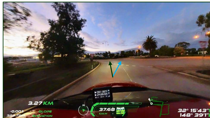
F1.3: Blueridge Dr southern approach leg looking north through the roundabout. The Blue arrow provides the approximate path of a speeding vehicle; the dark Green arrow approximates the prescribed travel path. (Image: WaySafe 2024.)
