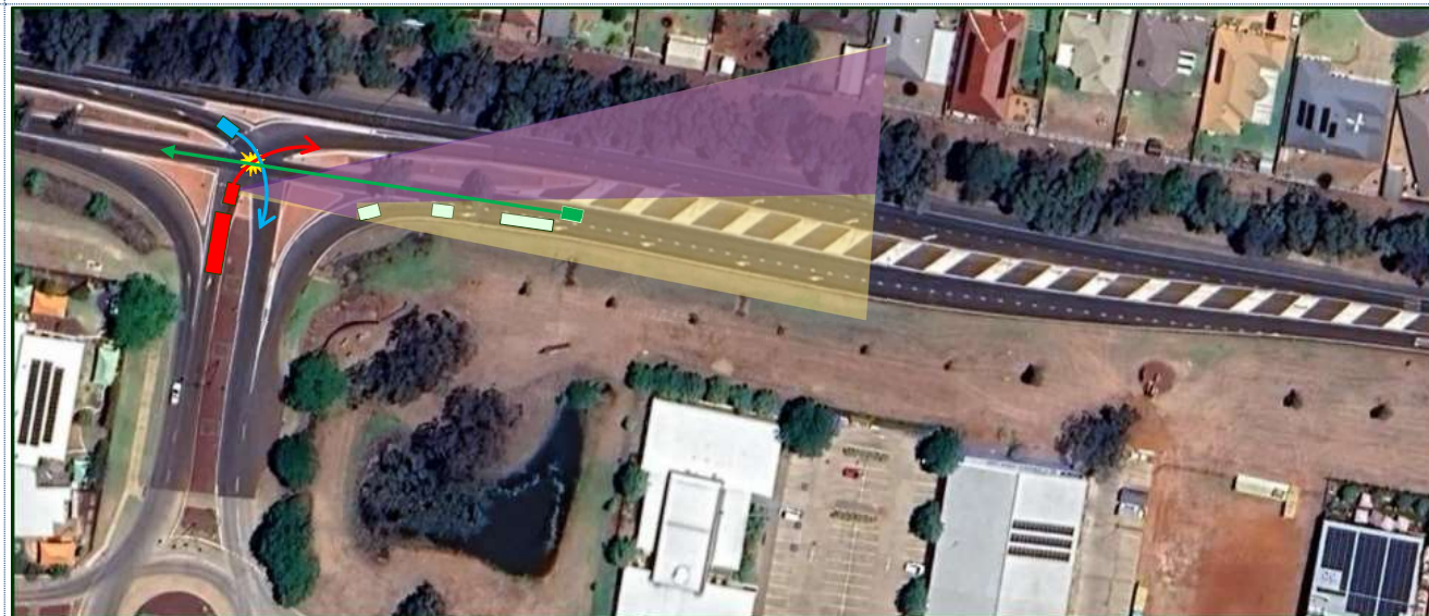
F7.1: Sighting limitations and potential crash types at a seagull T-junction.
