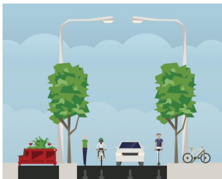
Typical Shared Zone Cross Section
