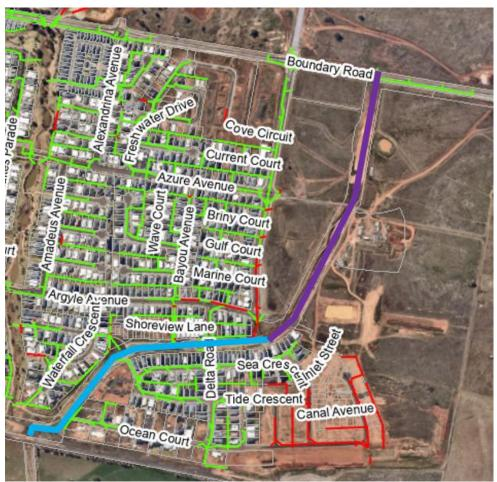
**Figure 3:** Extent of completed drainage channel within the drainage reserve indicated in blue. Extension required as part of this development application indicated in purple.
