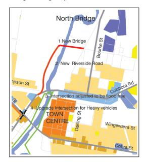
Figure 2.1 North Bridge and Highway Works
