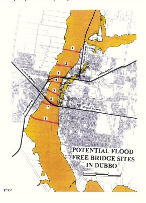
The map on the previous page shows the 1 in 100 year floodplain through Dubbo. On it are shown in red ALL the feasible locations for a new bridge to be built which would be "flood free" (ie, not inundated in floods smaller than the 1 in 100 year flood). The locations chosen are all somewhere near the CBD for obvious economic and social reasons – a bridge too far "out of town" would simply be an expensive white elephant 99.95% of the time when the river is not flooding.
