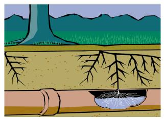
Figure 1. Tree roots seeking out moisture in a sewer pipe
