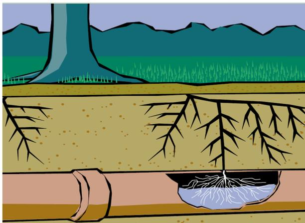
Figure 1. Tree roots seeking out moisture in a sewer pipe
