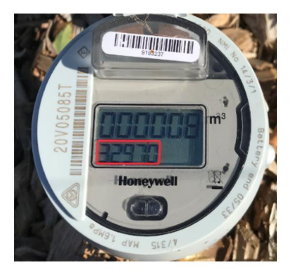
Top line displays Kilolitres. **Reading shown is 8 m3 which is equivalent to 8 kilolitres.**
